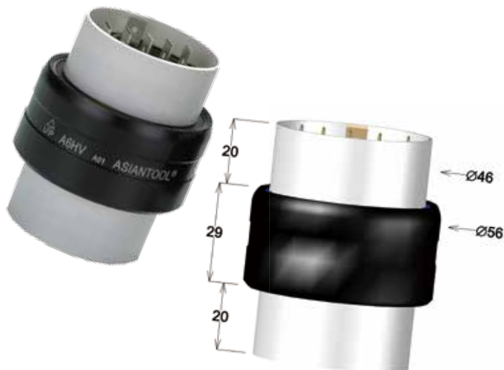
A6HV 6poles/30A/AC500V
