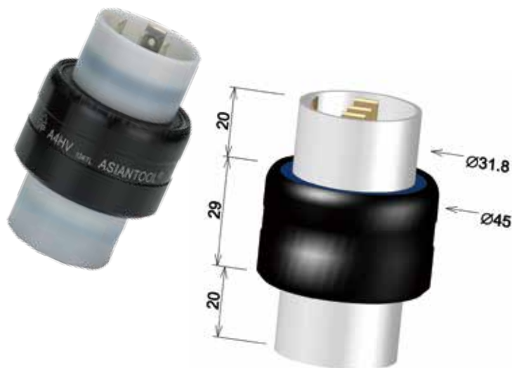
A4HV 4poles/30A/AC500V
